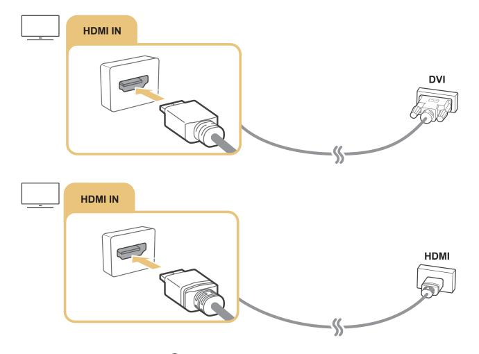
When you have connected a PC, go to (a) > > Source, and then select the PC icon from the external device icon list. For more information about the port settings, refer to "Editing the name and icon of an external device".
