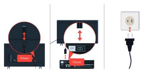
First disconnect and reconnect the power cables and HDMI cables on the back of your TV or the One Connect (OC) Box, then unplug the power cable and plug it back into the wall outlet.
