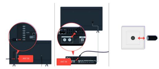
Check the antenna and input cable connections.
