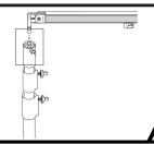
Connect the horizontal drape support to the top of an upright. Insert the pin into the slot, press the spring button to insert, then release it to lock.
